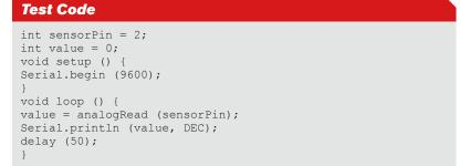
Testing the module's output analog voltage value, we find that when there is light, the output voltage is high, the equivalent of the switch being turned on. When there is no light, the output voltage is low, the equivalent of switched off.
